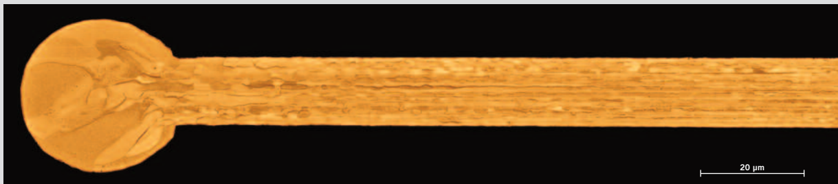
Cross-section of Fine & Short HAZ
